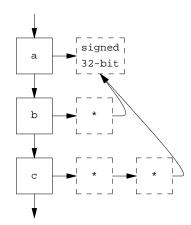
Lastly, the following diagram shows how an enumerated type is stored internally; it has a symbol table entry of its own so it can be found again in the future, similar to a structure definition.
