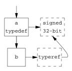
Here we see a special symbol table entry storing the type definition, and a second symbol table entry making use of the type definition via a type ref node.
